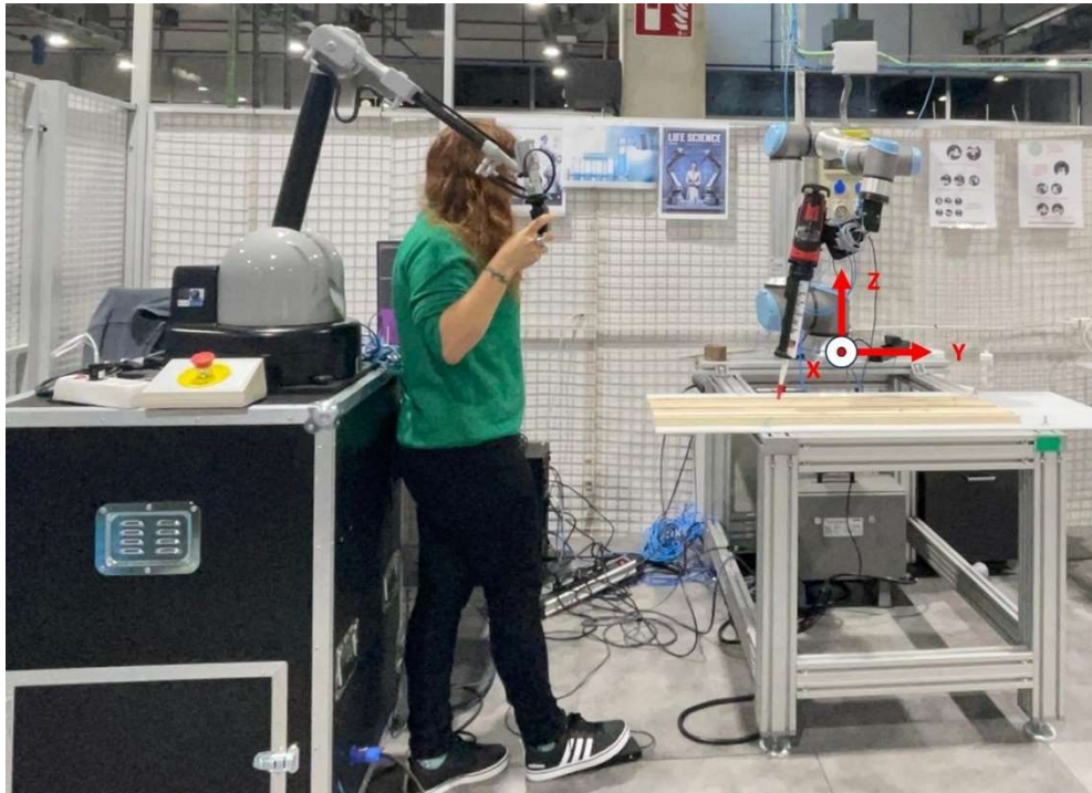
Figure 3 Frame reference (red) located at the base of the robot
