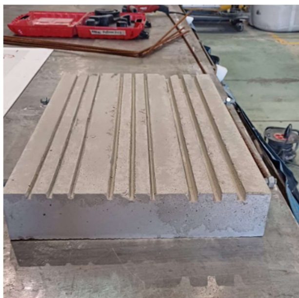
Figure 17 Real concrete block with 3 different joint sized built for user experiments
