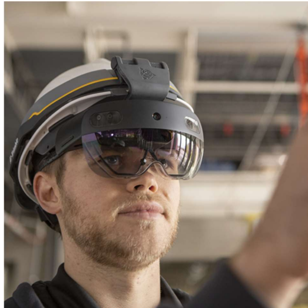
Figure 4 Trimble XR10 helmet - The only HoloLens 2 solution compatible with an industry-standard hardhat 9 and certified for use in safety-controlled environments.
