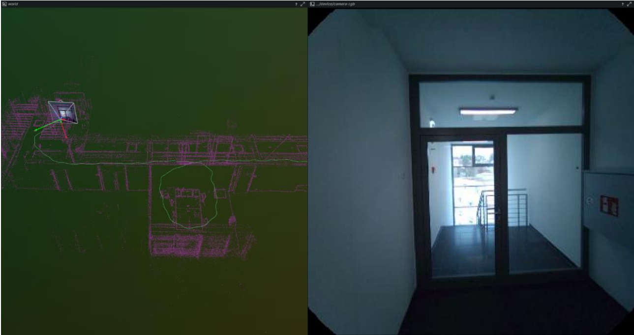
Figure 19 Display of interactive visualization of the Project Aria VRS RGB frames along with MPS data – Closed loop trajectory (in green), estimated semi-dense global point cloud (in purple) of DFKI hallway, and RGB image with estimated 6DOF pose.
