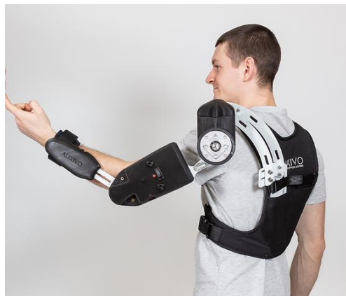
Figure 9 – EduExo Pro from Auxivo. This exoskeleton is the base of Humantech's exoskeleton.
