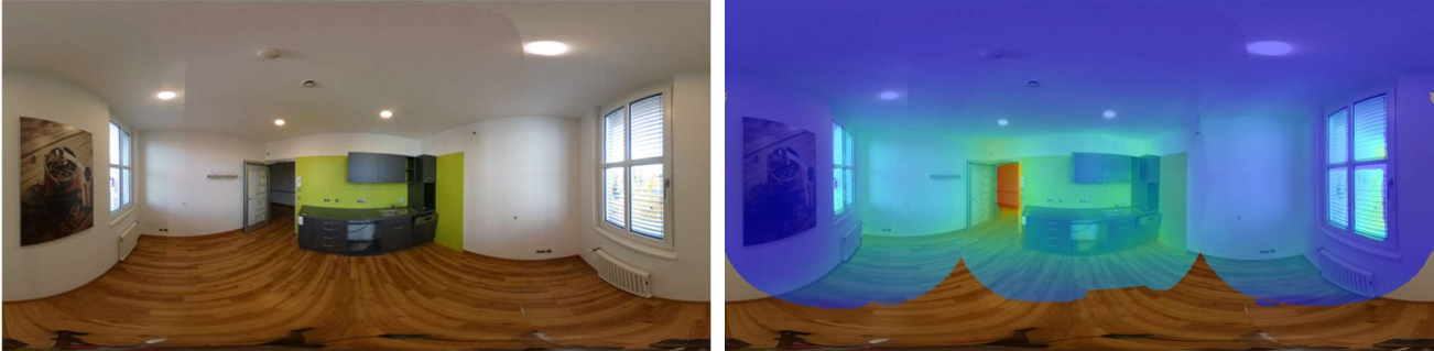
Figure 2 Left: An example of a panoramic image captured using the RICOH camera at the Weingarten site. Right: Depth measurements overlapped with the colour information showing the full RGB-D capabilities of the device
