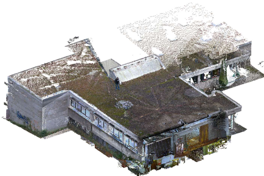
Figure 1 Example of a point cloud recorded by RPTU using the Leica BLK360 G2 at the Prot. Kirchengemeinde in Kaiserslautern
